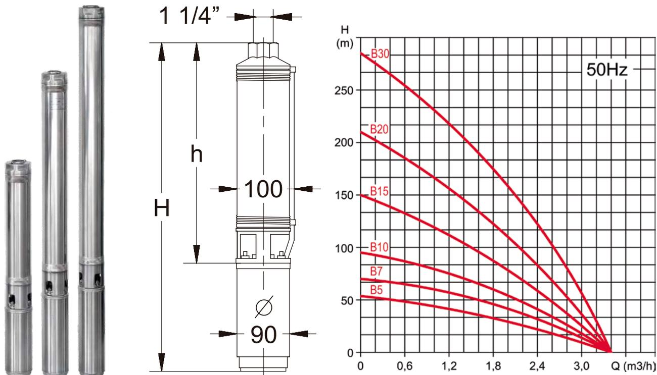
Selection curves: 2850 r / min, water at 20 ° C, according to ISO 2548 standard and C
