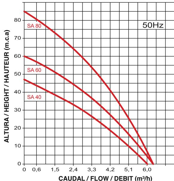
Curves at 2850 rev / min - Temperature 20 °C
